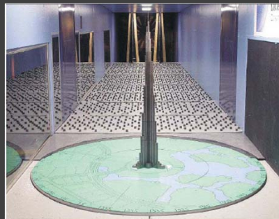
a) Aeroelastic Model at 1:500 scale
